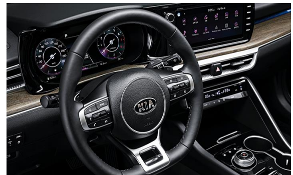
Fig 6: VR design quality assurance process had a major role in resolving the light reflection issues of the metallic and high-glossy material used for the K5's interior (Source : metrology.news)
